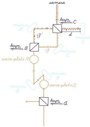
FIG. 1: Via the first two mirrors, the laser beam is aligned parallel to the optics table and the holes in the optics table. It diverges and reconverges following the classic Mach-Zehnder setup until beamsplitter C, where the upper path P' transmits through, then is reflected by, beamsplitter C. The waveplates attenuate the beam and allow for adjustment of the relative path intensities.
