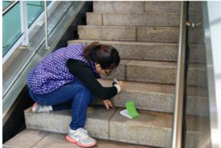
Figure 16 Measuring the Height of the Stairs
